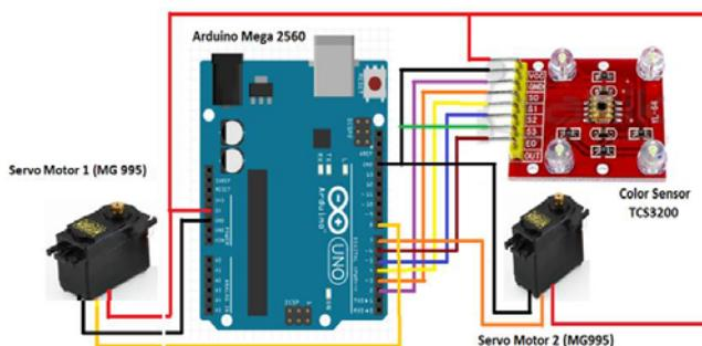
Fig. 6. Connection set up for the Color Sorter
