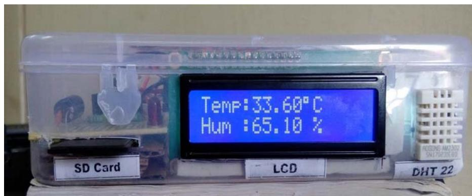
Fig. 12. Overall setup of the designed data- logger
