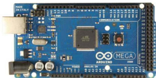
Fig. 1. Arduino Mega Board
