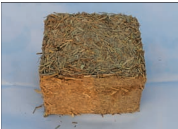
Feed block made of paddy straw and DDGS with optimum combination
