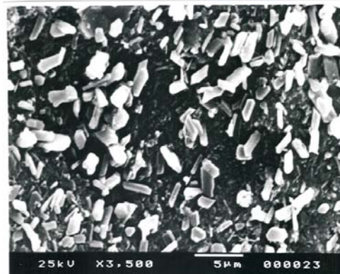
Scanning electron micrograph of chrome tanned mithun hide surface at 3500X magnification
