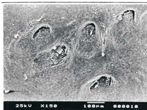
Scanning electron micrograph of chrome Tanned cattle hide surface at 150X magnification (wet blue tanned)
