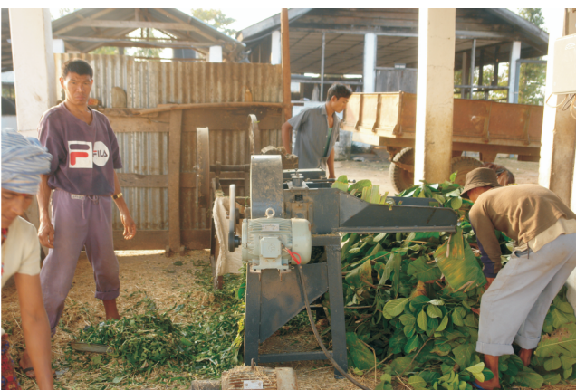
A newly installed chaff cutter in farm operation
