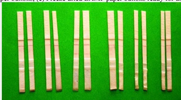
Visualization of species-specific paper based LAMP-LFA assays (Single line -Negative, Double line- positive)
