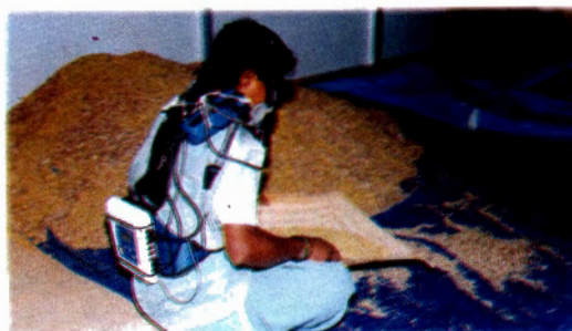
Measurement of heart rate and oxygen consumption of women worker using metamax energy measuring equipment
