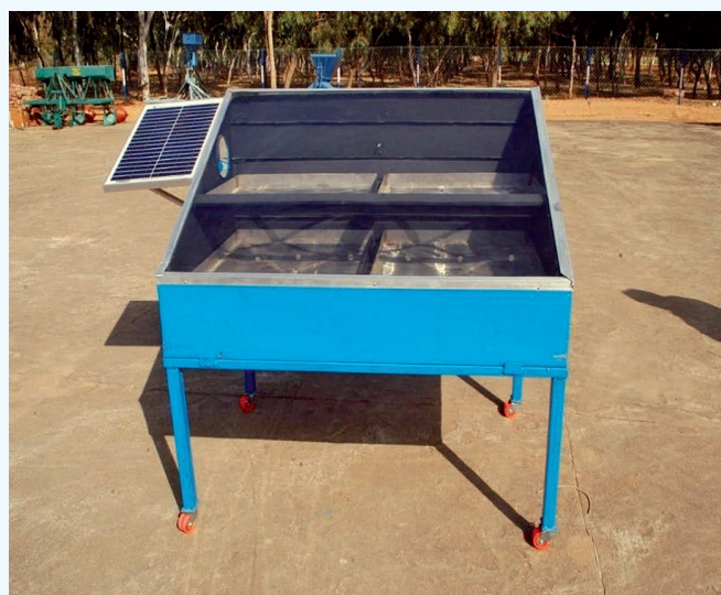
PVT hybrid solar dryer installed at CAZRI solar yard
