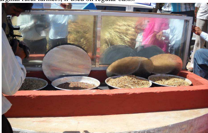
Fig. 1: Animal Feed Solar Cooker
