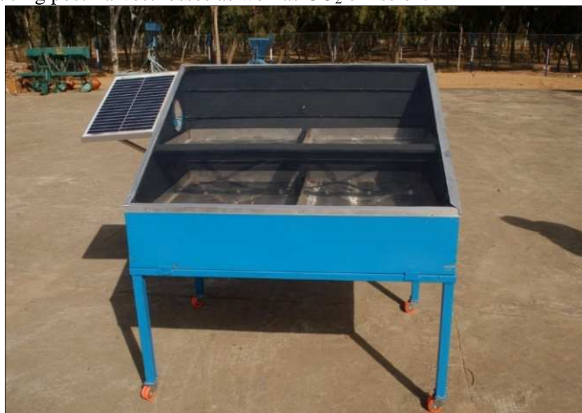
Fig. 7: PCM based PVT hybrid solar dryer
