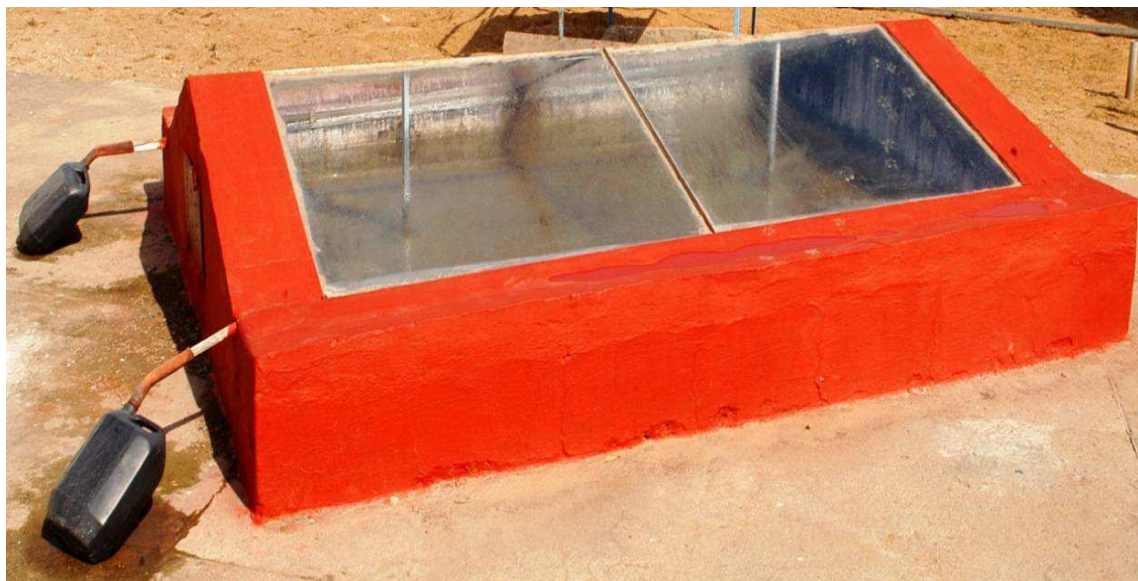
Fig. 8: Solar Desalination Devices Made of Vermiculite-Cement Plastered Material
