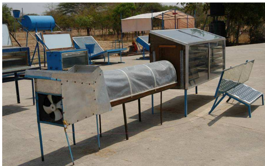
Fig. 5: PV Winnowing-cum- solar Dryer
