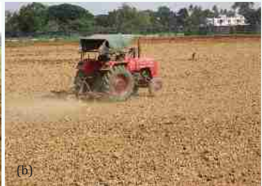
Plate 1. Field preparation using tractor drawn mould board plough (a) and cultivator (b) for dry direct sowing of rice
