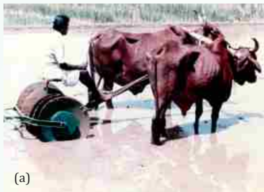
Plate 5. Puddling operation using animal drawn disc harrow (a) and tractor rotavator (b)
