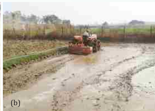
Plate 5. Puddling operation using animal drawn disc harrow (a) and tractor rotavator (b)
