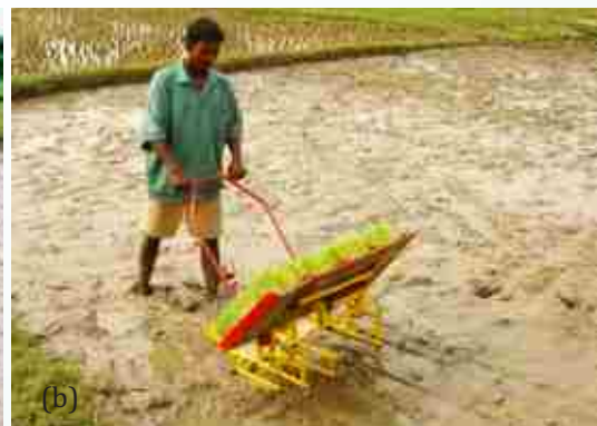
Plate 6. Transplanting of rice by 8 row mechanical transplanter (a) and four row manual transplanter (b)
