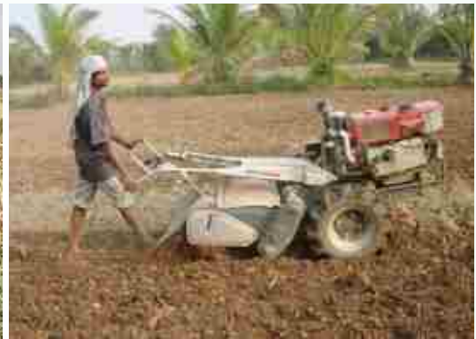
Plate 2. Field preparation using power tiller for dry direct sowing of rice
