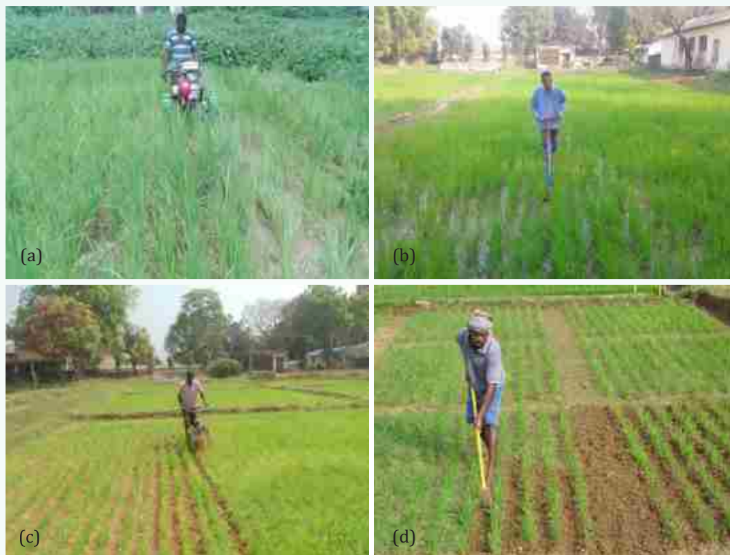
Plate 8. Weeding in rice with different mechanical weeders power operated two row wet land weeder (a) star cono weeder (b) power operated single row dry land weeder (c) & finger weeder (d)
