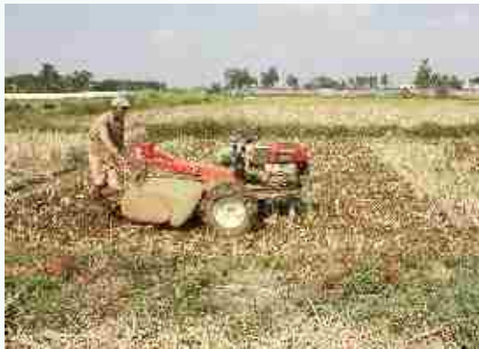
Plate 2. Field preparation using power tiller for dry direct sowing of rice
