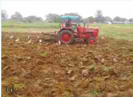
Plate 1. Field preparation using tractor drawn mould board plough (a) and cultivator (b) for dry direct sowing of rice
