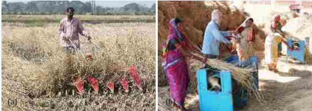
Plate 10. Harvesting by reaper (a) and threshing by electric drummy thresher (b)
