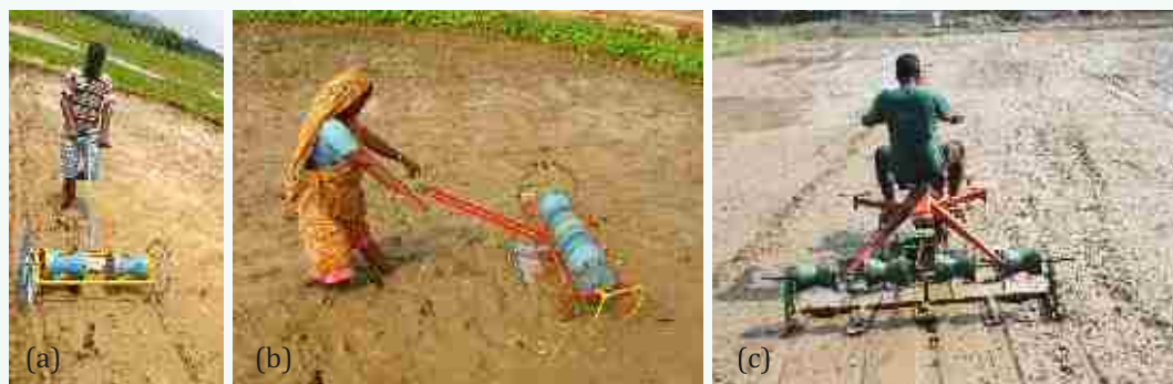
Plate 7. Sowing of pre-germinated seeds with manual four row drum seeder (a), manual six row drum seeder (b) & power operated eight row drum seeder (c)
