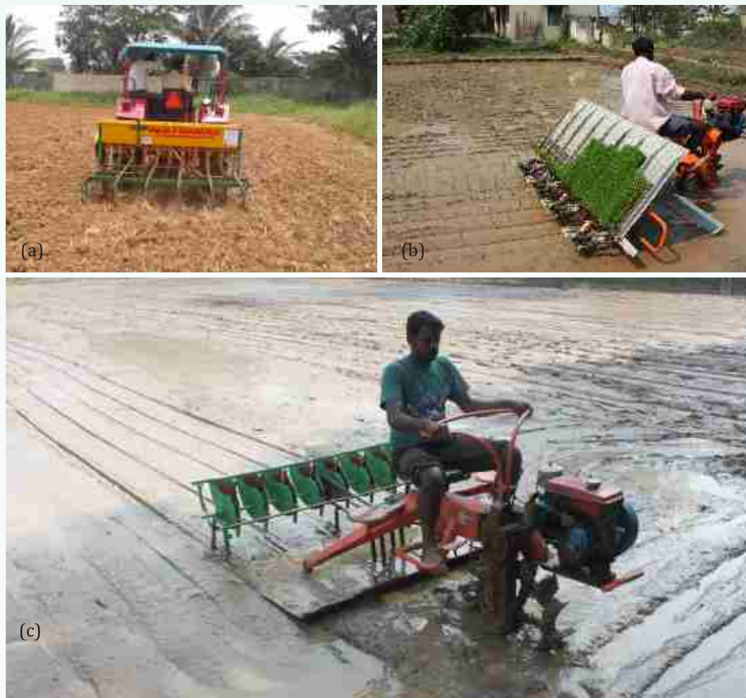
Plate 11. Sowing/planting under different establishment methods (a) dry direct sowing (b) transplanting (c) wet direct sowing used in the experiment
