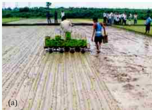
Plate 6. Transplanting of rice by 8 row mechanical transplanter (a) and four row manual transplanter (b)
