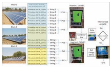
Fig. 3. Schematic diagram of PV based electricity generation in agri-voltaic system and its supply to local grid.
