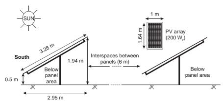
Fig. 2. Design of typical agri-voltaic system.
