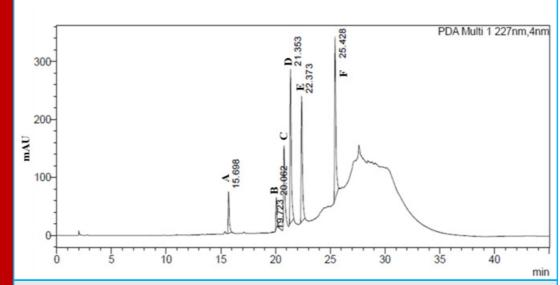
FIGURE 1D. Standard HPLC chromatogram of extracts of W. somnifera roots. A.Withanoside IV (Rt=15.69), B. Withanoside V (Rt=19.72), C. Withaferin A (Rt=20.06), D. 12-Deoxy Withastramonolide (Rt= 21.35), E. Withanolide A (Rt=22.37), F. Withanolide B (Rt=25.42)
