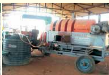
Urea solution spray attachment fitted to thresher
