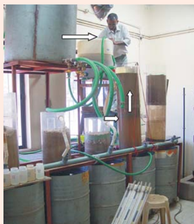
Laboratory set-up for testing efficiency of filter system comprising gravel, sand and agro-net in case of upward flow of runoff through filter system
