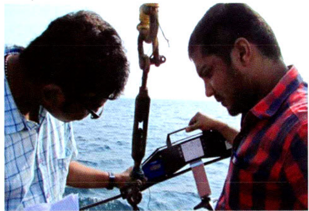
Warp tension meter in use
