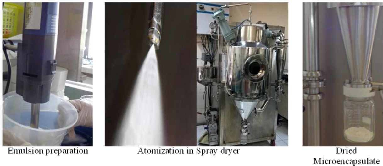
Fig. 2 Microencapsulation process by spray drying
