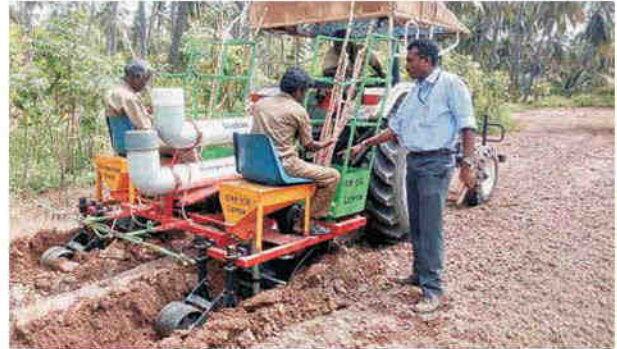
Fig. 35. Evaluation of IISR-Sugarcane Cutter Planter at TNAU, Coimbatore
