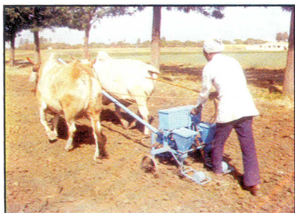
Fig. 18: Seed-cum-fertilizer drill with pair of bullocks
