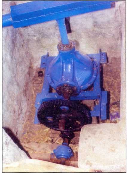
Fig 1. Rotary mode transmission gear unit established at Balaji Camp
