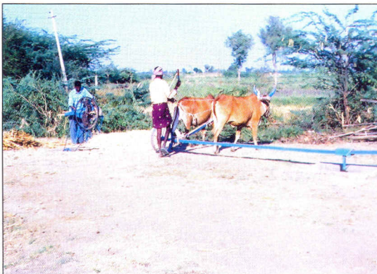
Fig 2. Chaff cutting operation of jowar fodder stalk at Balaji camp
