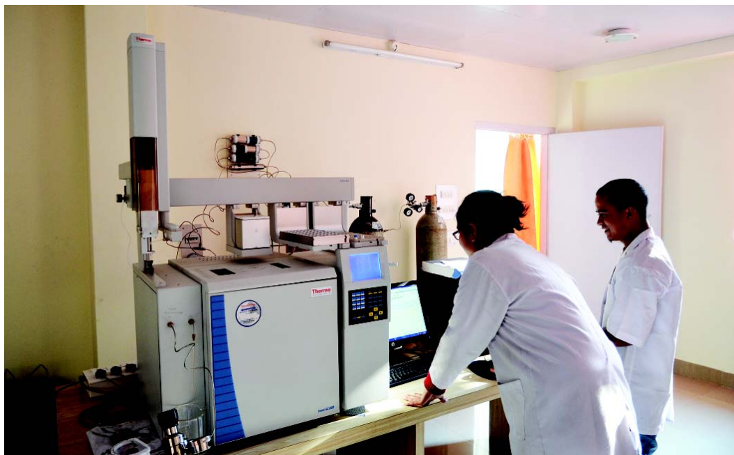
Gas chromatography installed in central lab of ICAR RC NEH, Umiam, Meghalaya
