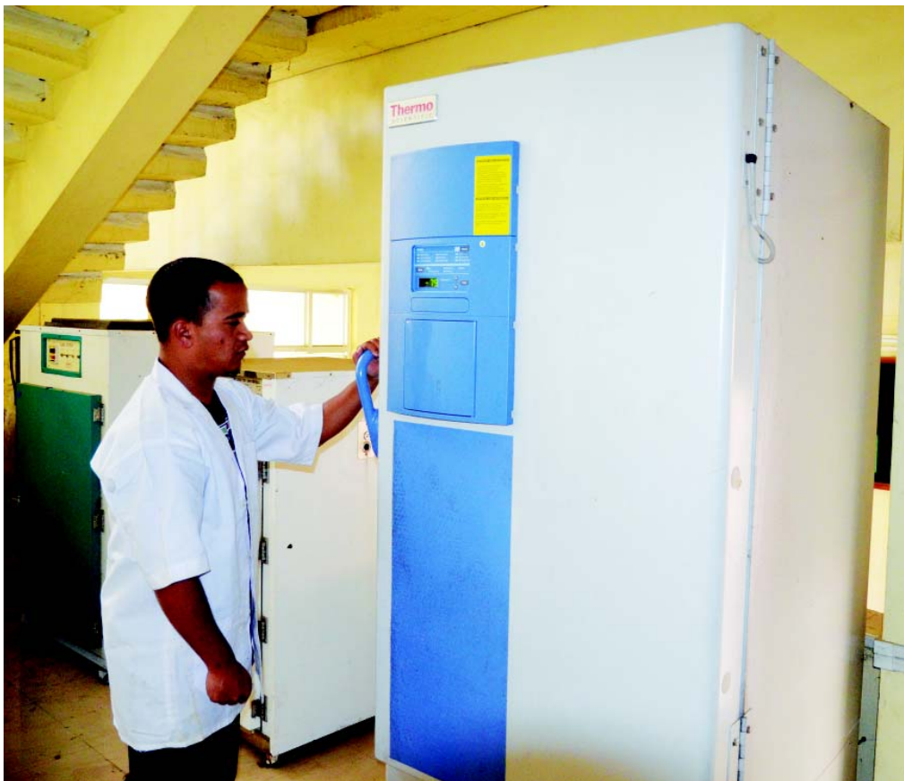
Ultra deep freezer is used for storing plant and animal tissues for long time under very low temperatures
