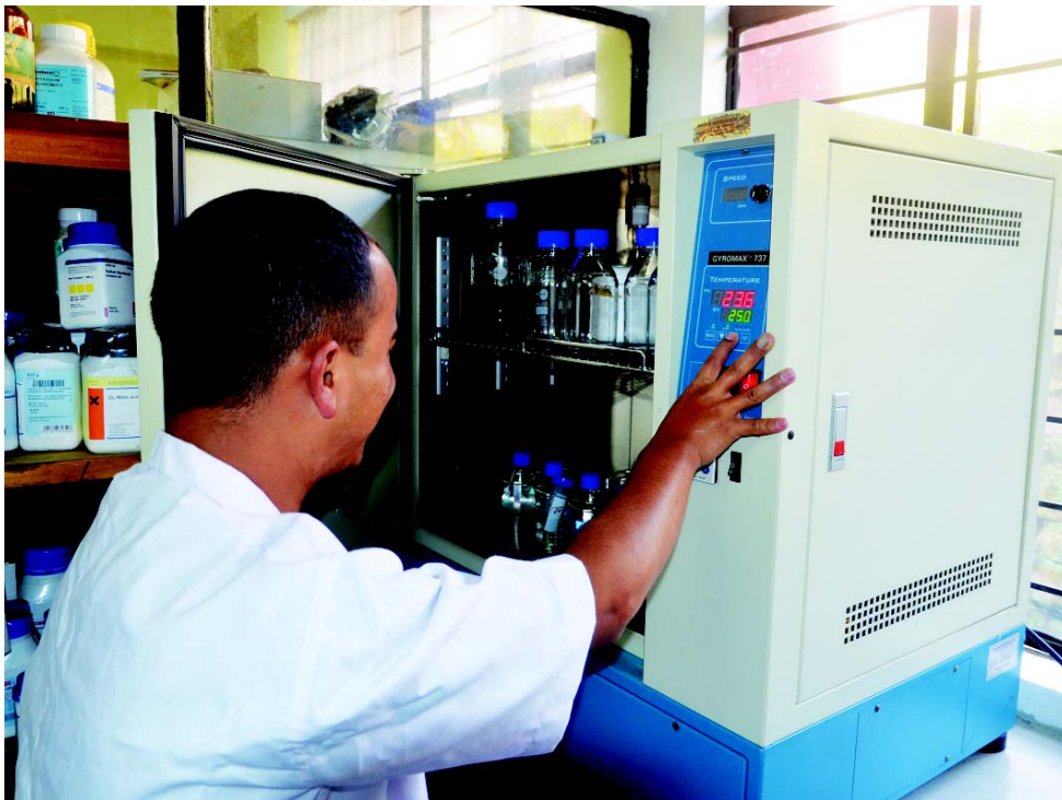
Controlled Environmental laboratory shaker used for incubation and shaking of biological samples under desired temperature and light conditions
