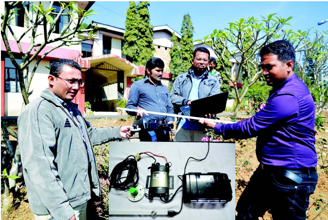
Line quantum sensor components and light intensity measurements near plant canopy
