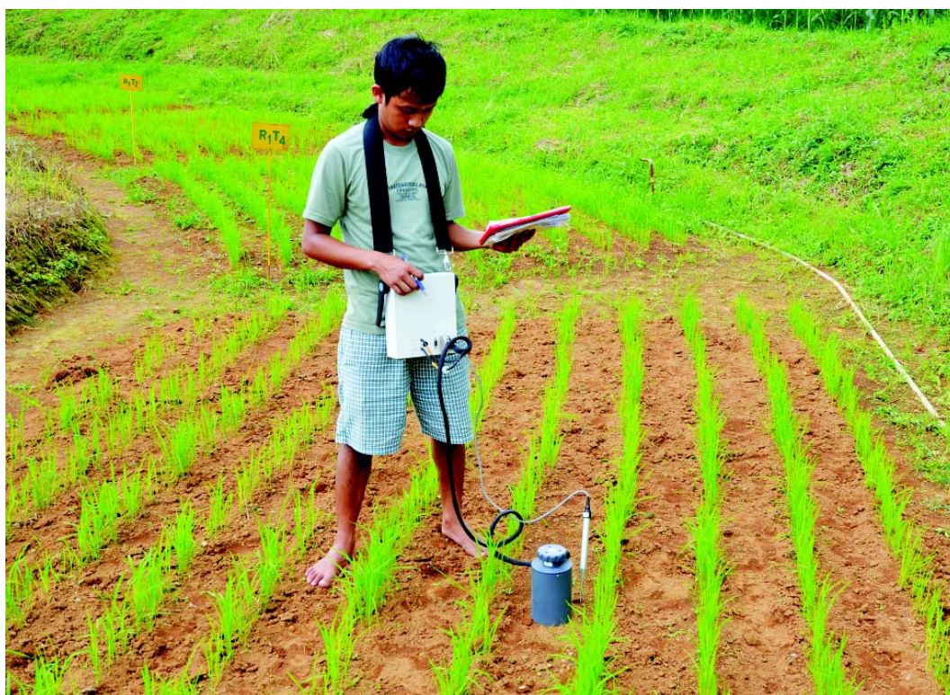
EGA measurements in dry seeded paddy field
