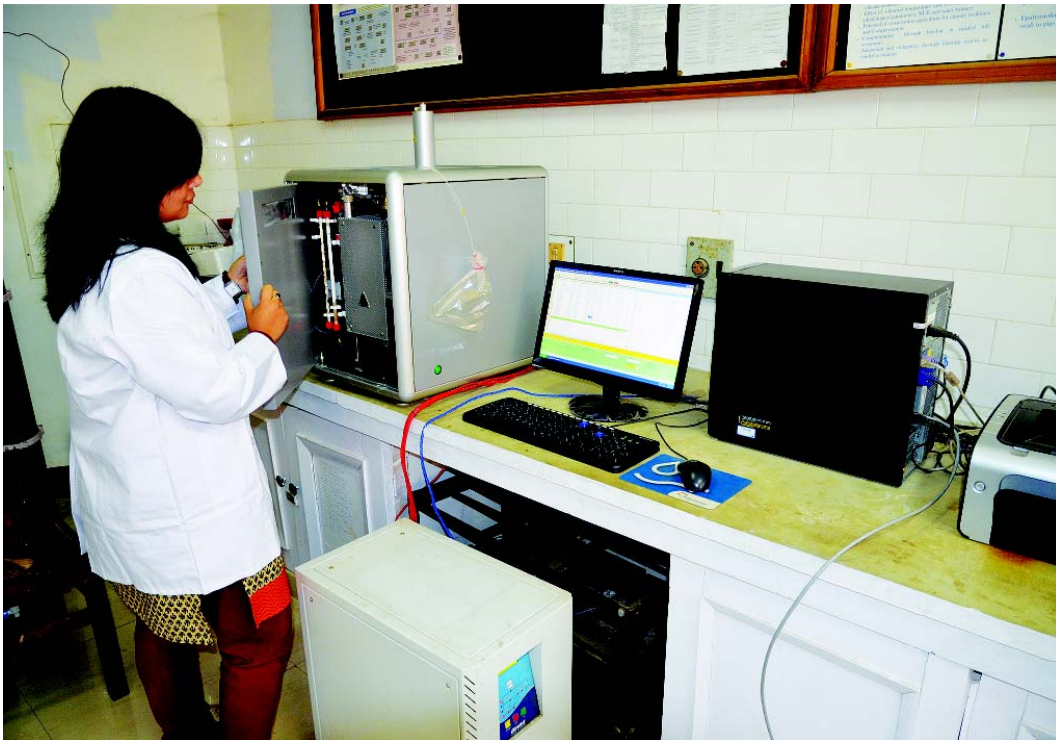
General view of TOC Analyzer connected with TIC Module
