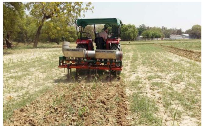
Fig. 5.3. Multipurpose tool frame with interculturing attachments
