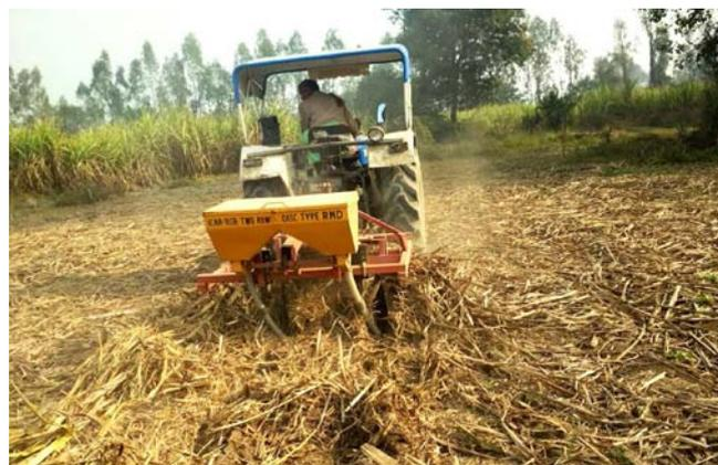
**Fig.5.5. Two row disc RMD with stubble shaving attachment**
