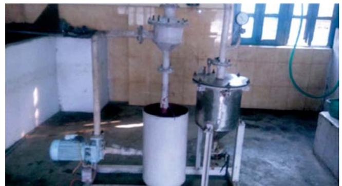
Fig. 6.2. Molten jaggery pumping device
