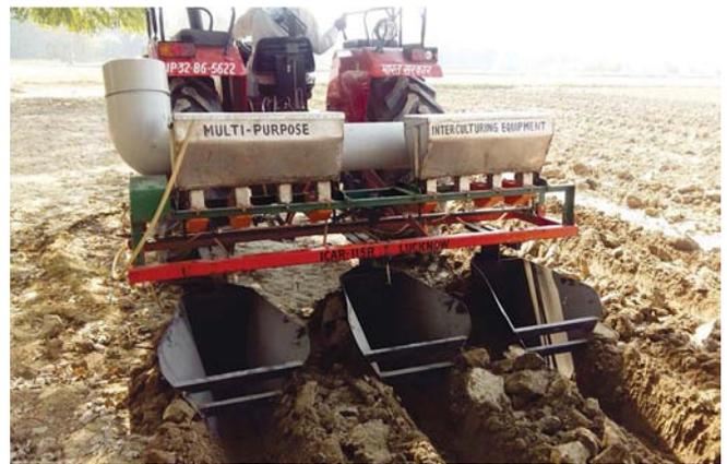
Fig. 5.2. Multipurpose tool frame with furrow opening attachments
