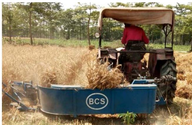
Fig. 5.8. Tractor operated reaper binder in field operation for wheat harvesting
