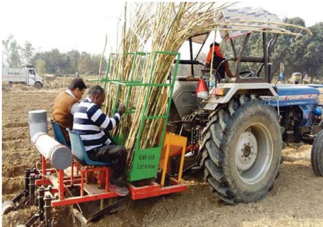
Fig. 5.1. Field demonstration of newly developed planter at farmers' field.
