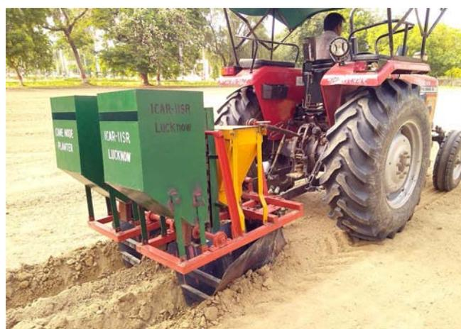
**Fig. 5.6. Tractor operated cane node planter in field operation**
