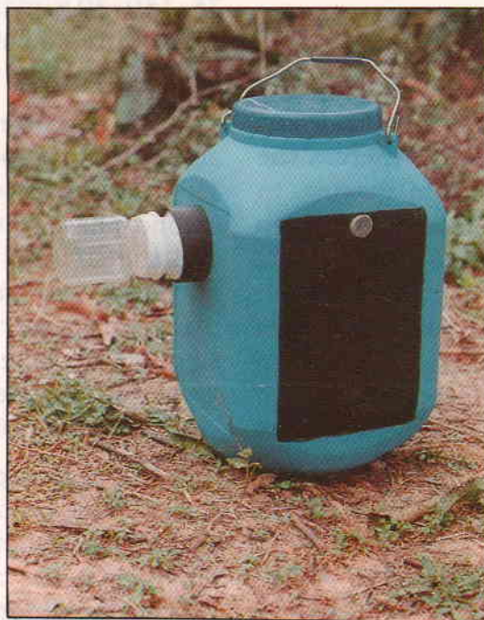
Device for separation of lac-associated insects
