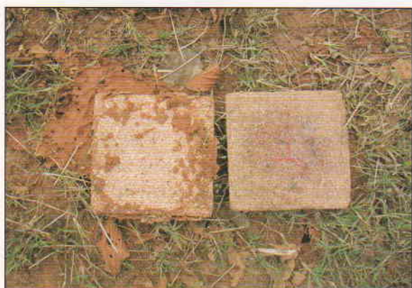
Fig.45. Termite resistance behaviour of sticklac composite board (a) control (b) with 2% chlorpyrifos
