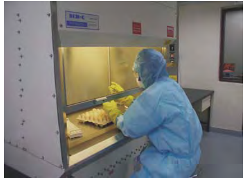
Personal safety is an important component of biosafety, A lab worker having personal protective equipment is carrying out AI virus inoculation
