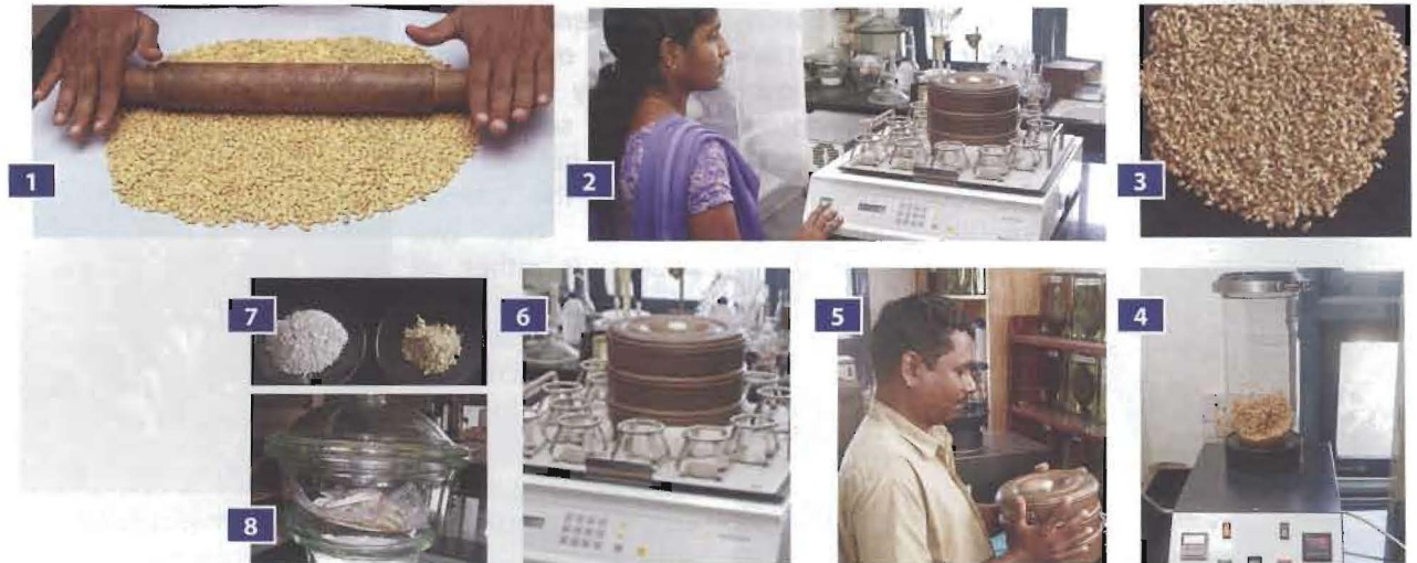
1 Fig. 6. Crushing mature male flowers 2 Fig 7 Drying male flowers in incubator 3 Fig. 8. Dried male flowers 4 Fig.9. Drying male flowers in fluid bed 5 Fig.10. Manual sieving of male dried flowers 6 Fig.11. Sieving of dried male flowers 7 Fig. 12. Pollen and talc for preparation of pollen-talc mixture 8 Fig 13 Processed pollen stored in desicator
