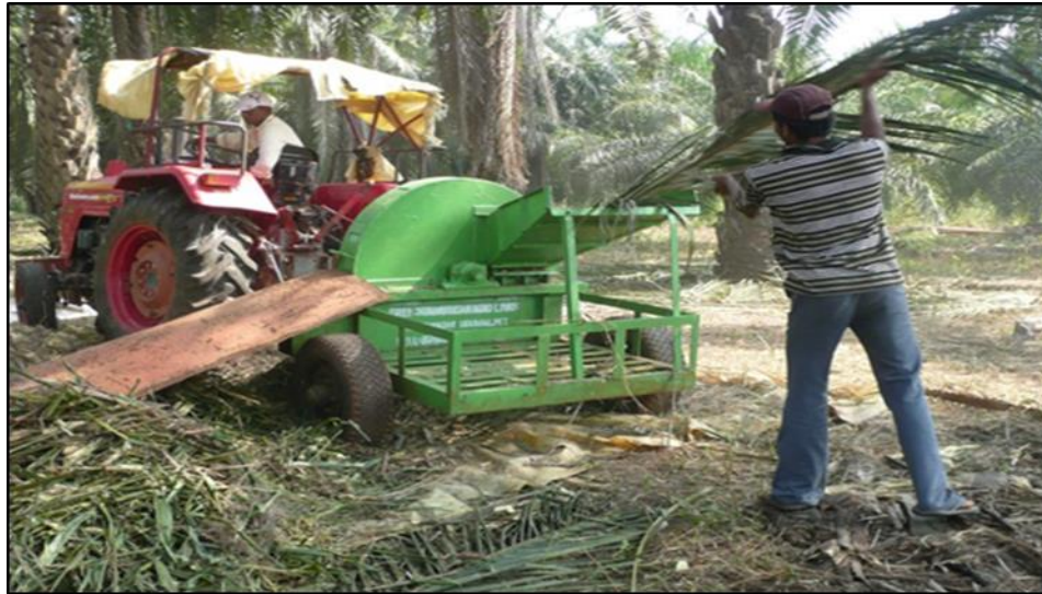
Figure 1. Chopping of palm leaves with the help of tractor driven shredder machine
