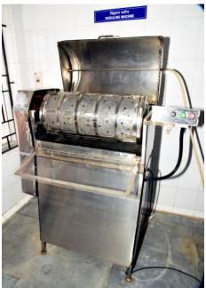
Fig.6 Fish de-scaling machine with variable drum speed
