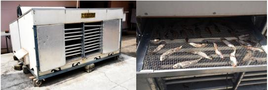
Fig.5. CIFT Solar-Cabinet Dryer with Electrical back-up
