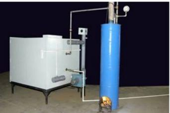
Fig.3 CIFT Solar-Biomass Dryer
