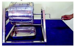
Fig. 7 Fish de-scaling machine hand operated
