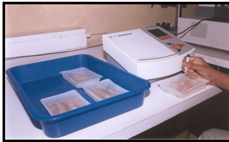
Fig 2. Modified Atmosphere packaging equipment and Gas composition analyser
