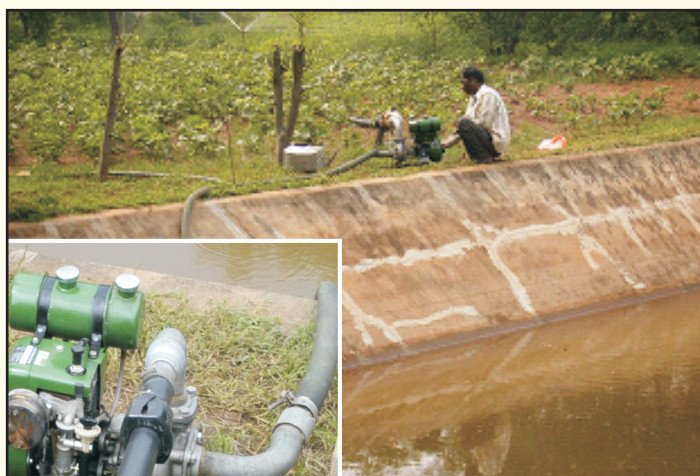
Portable pump in operation for lifting water farm pond and sprinkler irrigation
