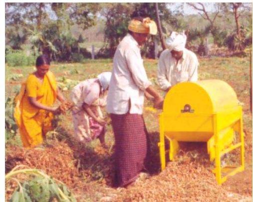
Fig. 18. Groundnut stripper in farmer's field
