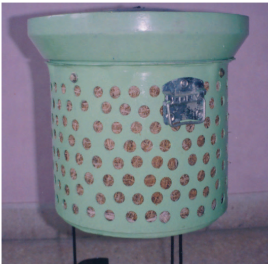
Fig. 19. Vegetable preservator (5 kg capacity)
