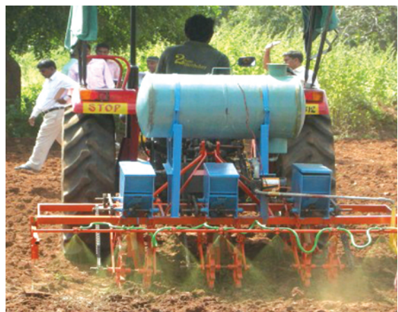
Fig. 7.Precision planter cum herbicide applicator
