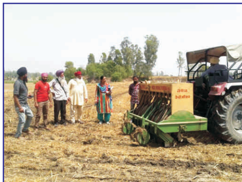
Demonstration on working of Happy Seeder
