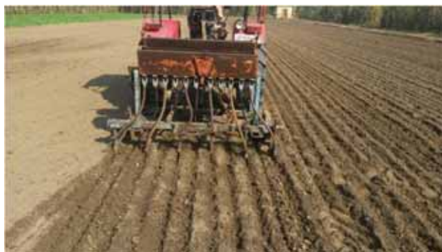
Plate 29: Line sowing of mustard using seed drill
