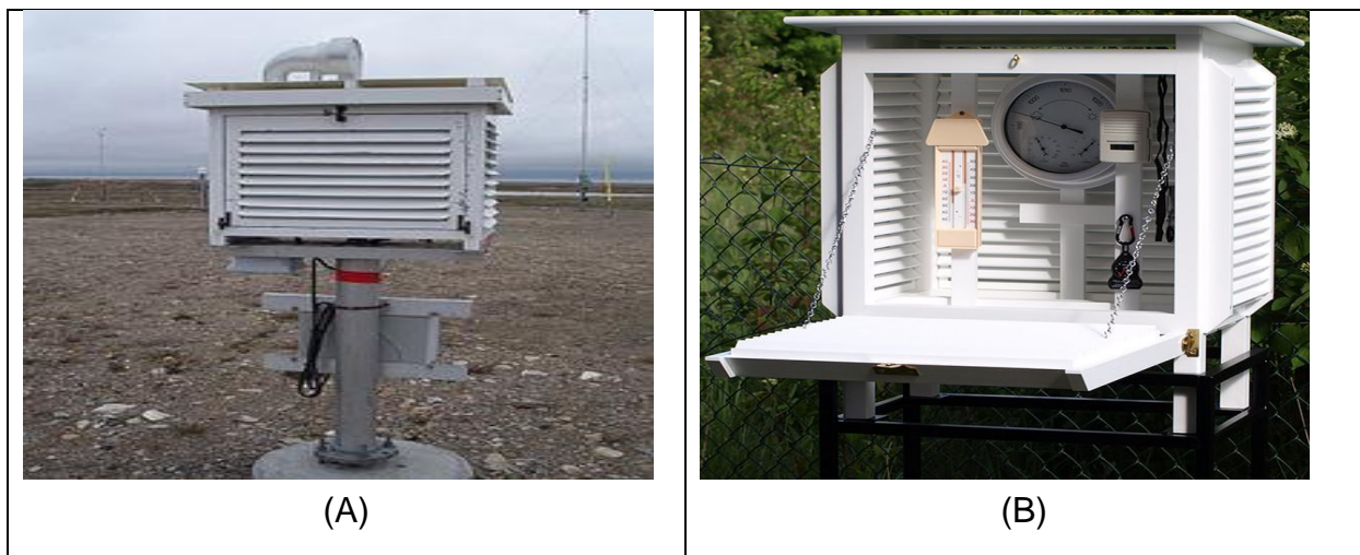
Fig 4. (A) Outer view of Stevenson screen , (B) inner view of Stevenson screen
