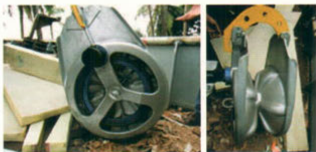
Indigenously fabricated power block ready for installation on-board steel trawler
