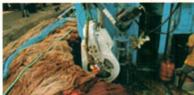
Chinese power block installed in purse seiner at Goa
