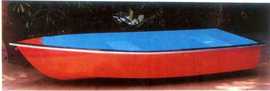
The 3.5 FRP row boat specified by CIFT for fishing in Thariode and Pookot lakes of Wynad District
