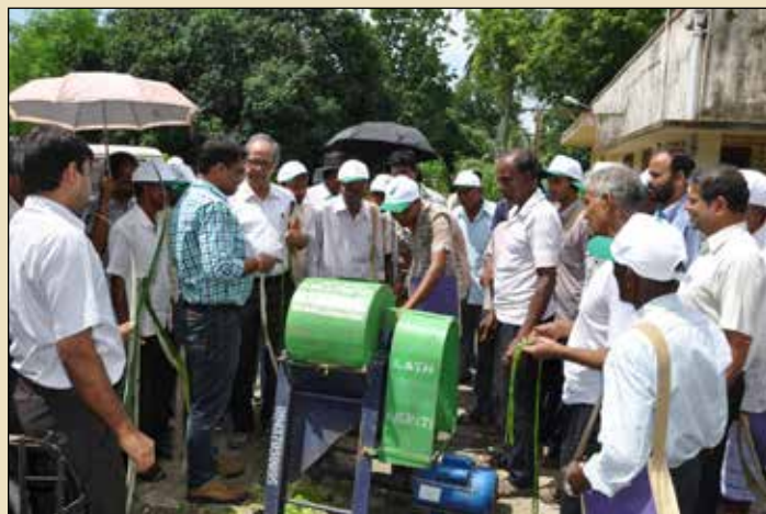
Er. R.K. Naik demonstrating sisal fibre extraction using sisal fibre extractor
