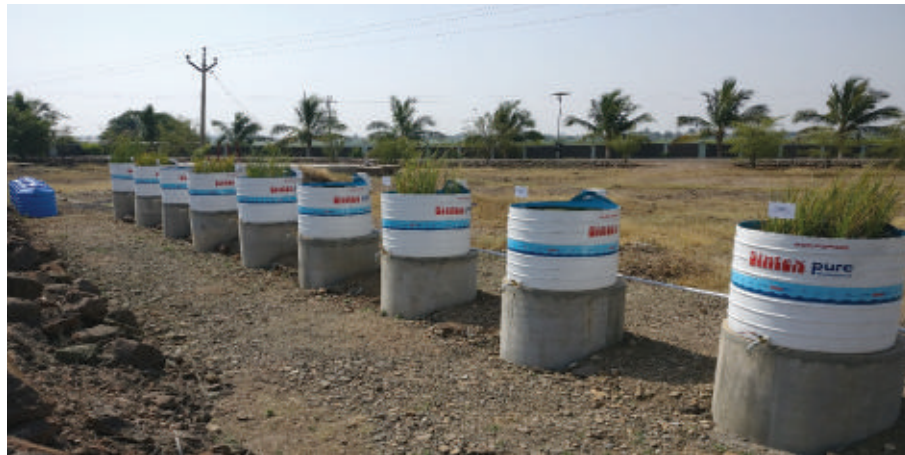
Fig. 2.29. Experimental vertical sub-surface flow constructed wetland system (HSSF-CWs)
