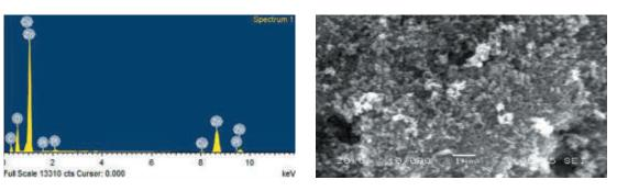
Fig. 2.27. SEM photograph of prepared zinc oxide nanoparticles
