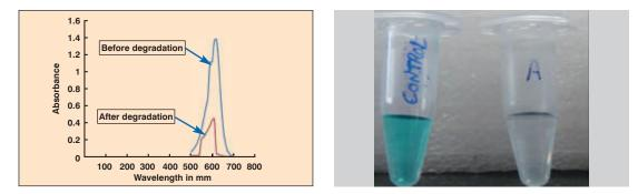
**Fig. 2.28.** Photodegradation of malachite green by zinc oxide nanoparticles with and without zinc oxide nanoparticles
