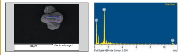
Fig. 2.29. SEM photograph of biologically synthesized selenium nanoparticles EDS spectra of biologically synthesized selenium nanoparticles
