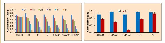
Fig. 2.26. Ammonia removal activity of native zeolites and heulandite and silver ion exchanged heulandite with and without silver nanoparticles
