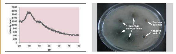
Fig. 2.30. XRD pattern of biologically prepared selenium nanoparticles antibacterial activity of selenium nanoparticles against *Aeromonas hydrophila* synthesized
