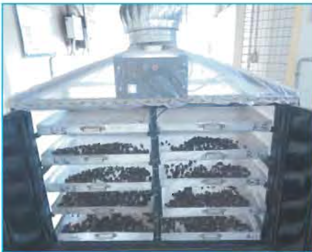
Multi-mode solar drier
