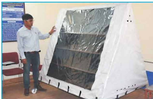
Solar based foldable tent dryer
