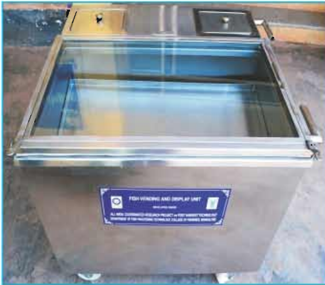
Refrigerated fish vending and display unit
