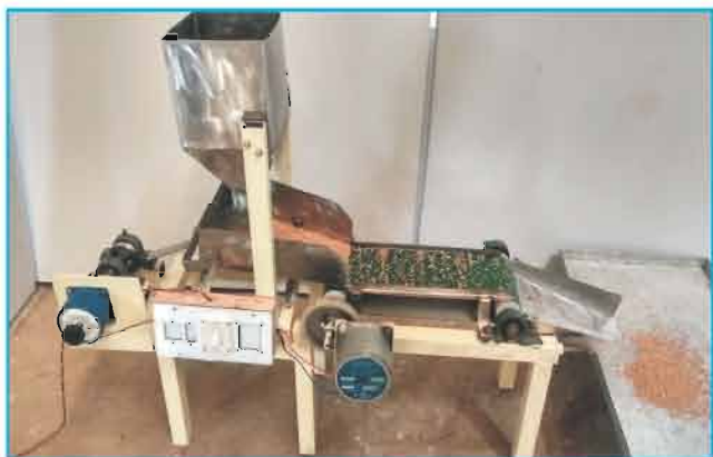
Prototype of smart device for automatic detection and identification of insects in stored grains
