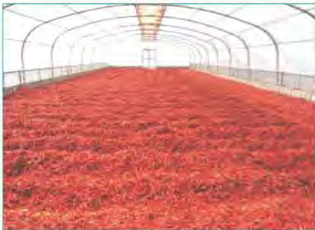
Modified ANGRAU polyhouse solar dryer for chillies
