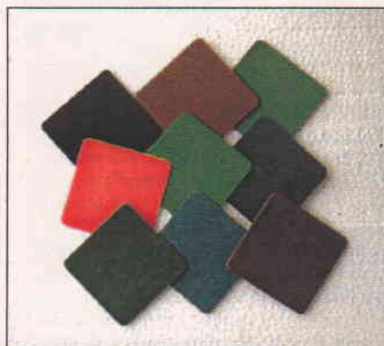
Tea coasters made of fibre glass reinforced sheets prepared with shellac-filled SMC
