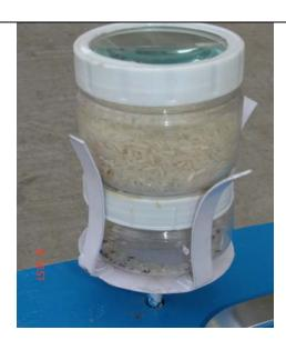
View of working of Mechanical device for detection of insects in stored grains Contributed by Dr. A. K. Thakur, Sr. Scientist (AS&PE), CIPHET, Abohar
