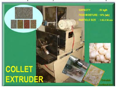
kg/h) and feed moisture (14%, wb), feed particle size (1.65-2.36 mm) were found optimum and kept constant for different protein enriched extruded snack foods. It is attached with a cutter (1 hp DC motor). The feed required particle size with predetermined formulation can be fed through feeder, which can be regulated by screw auger. The expanded products of 14-20 mm axial diameter can produced.
