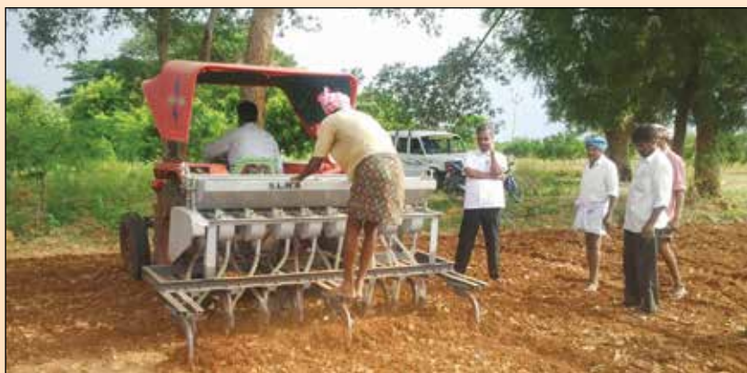
Sowing groundnut with Ananth seed drill
