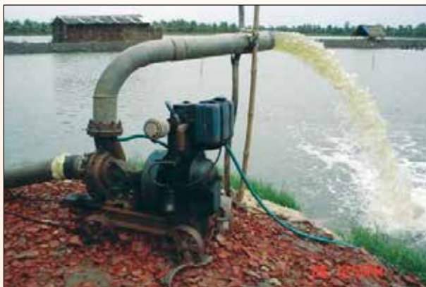
Recycling pond water to improve dissolved O 2 levels
