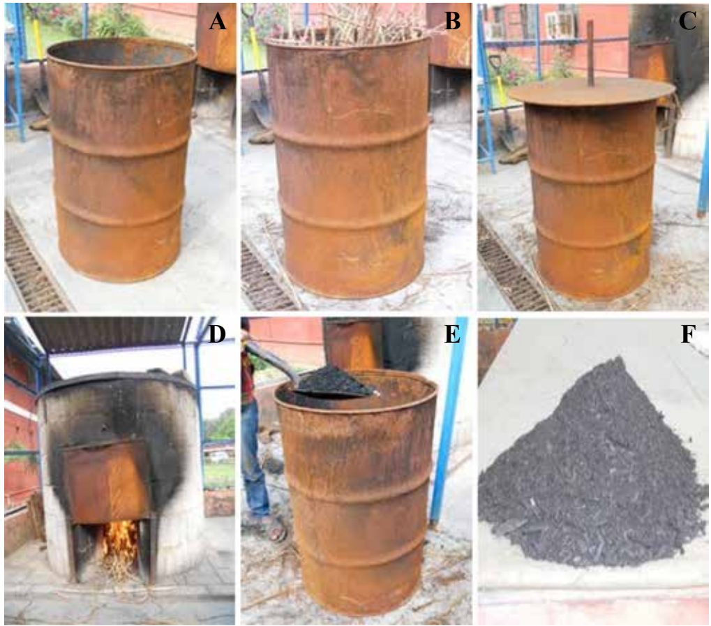
Biochar preparation at IARI: Drum used for preparation of biochar (A); Drum filled with maize stover (B); Drum covered with lid (C); Drum placed inside the firebrick kiln heating provide at the base of drum externally (D); Biochar removed from drum (F); and Biochar the final product with little percentage of ash (F)
