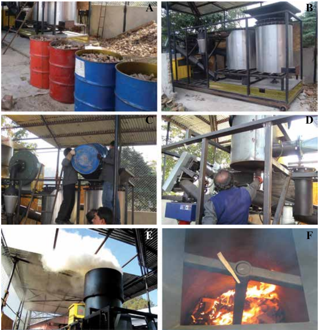
Biochar preparation using continuous biochar production unit at ICAR RC NEH, Barapani: wood chips collected in drums (A); continuous biochar production unit (B); feeding the biochar unit with wood chips (C); Firing the smoke with a torch (D); initial smoke from biochar unit (E); and wood chips burning inside main reactor (F)
