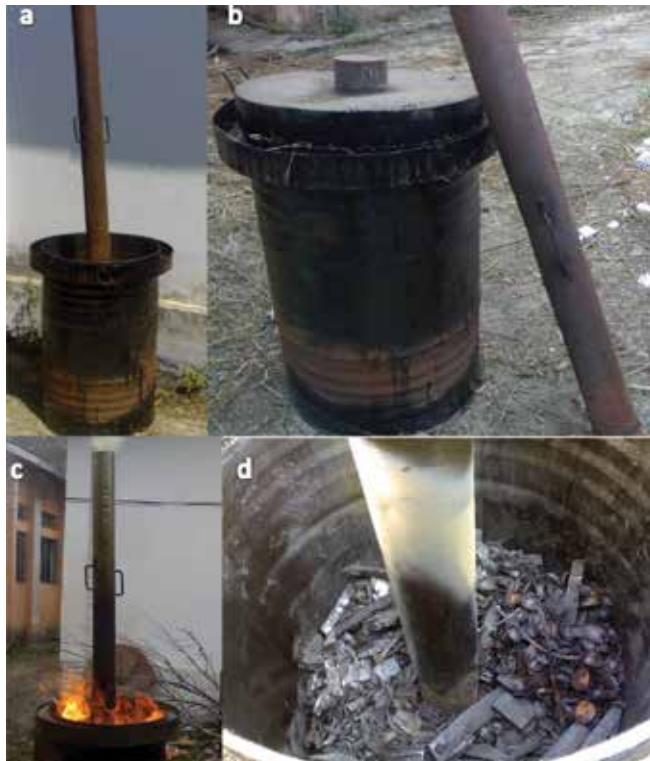
Portable metallic kiln (a) charring drum, (b) charring drum with lid and chimney, (c) burning of biomass during charring and (d) charred biomass after cooling
