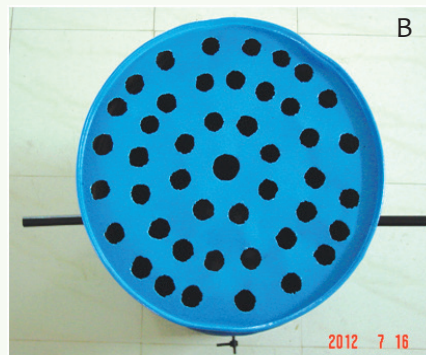
Fig. 4 : Low cost portable biochar kiln A. Whole assembly B. Bottom section
