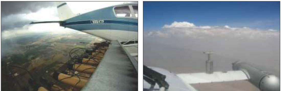
Fig 25: Flaring ejectors fitted to aircrafts releasing seeding material
