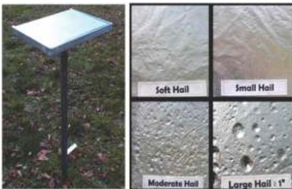
Fig 21 : Measurement of hail size using hail-pads
