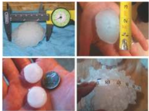
Fig 22: Different approaches to record the size of individual hailstone
