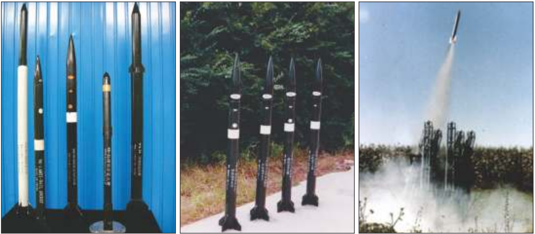
Fig 24: Anti hail rockets being fired from ground launcher
