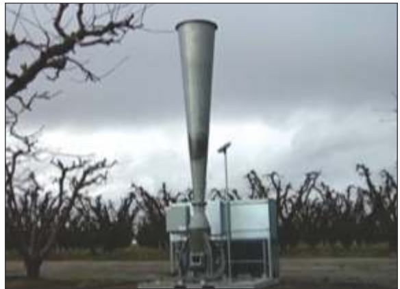
Fig 26: A hail control system in operation
