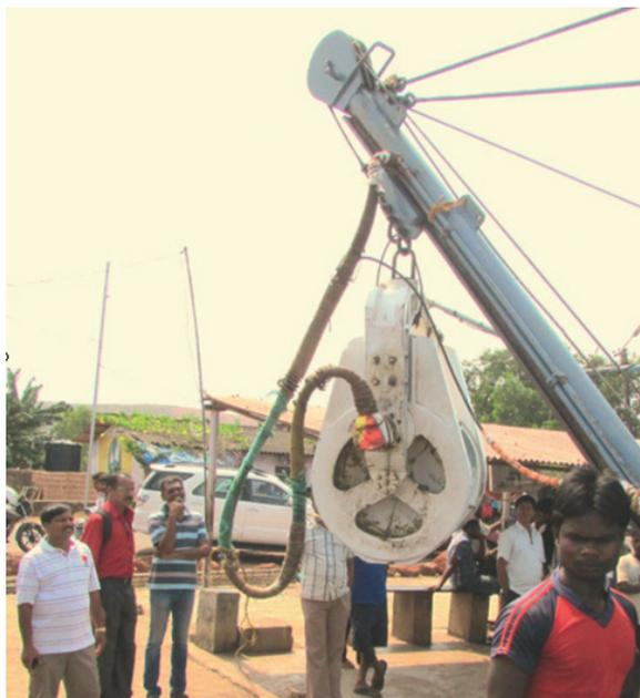
**Fig. 4. Power block used in purse seiners of Goa**
