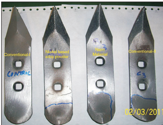
Control and coated Shovels after one hour of field operation
