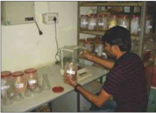
Fig 11. Weighing of soil samples by digital electronic balance and titration for organic carbon estimation
