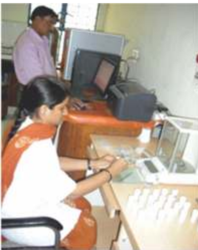
Fig 14. Handling of CHN analyser for estimation of total carbon
