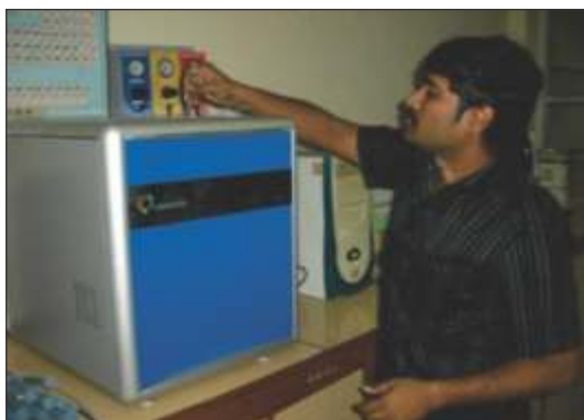
Fig 13. Handling of TOC analyzer for estimation of total carbon and inorganic carbon
