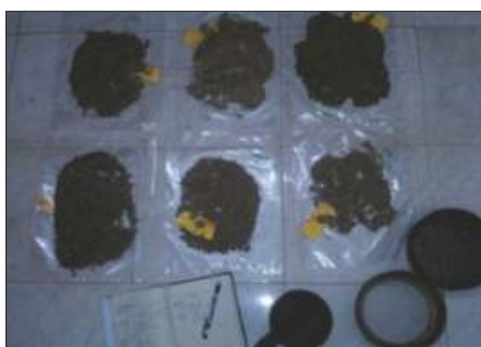
Fig 8. Soil sample air drying, processing and proper storage
