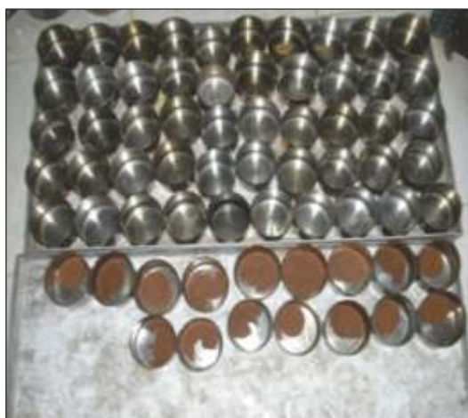
Fig 10. Collection of samples using core sampler and transfer of samples into cans
