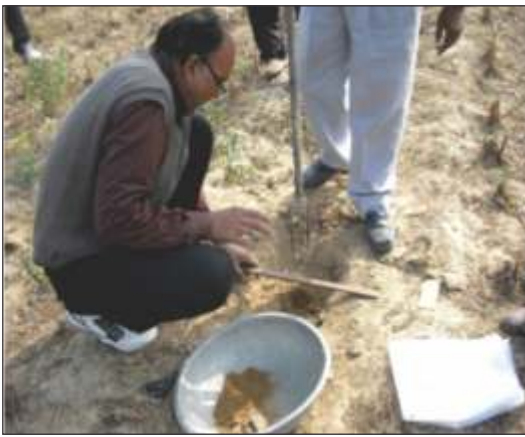
Fig 7. Collection of soil sample with (a) screw auger and (b) core sampler
