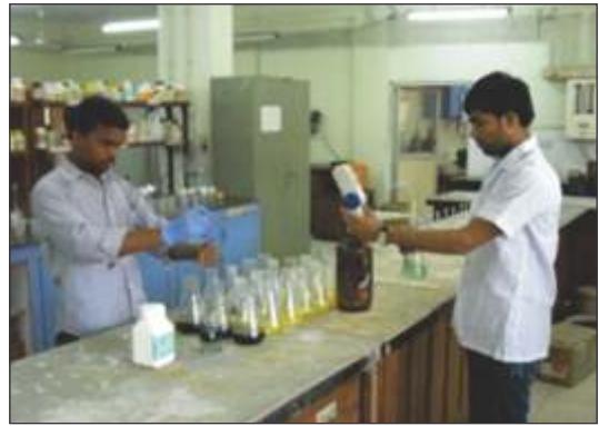
Fig 11. Weighing of soil samples by digital electronic balance and titration for organic carbon estimation
