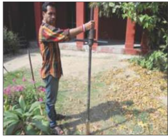
Fig 7. Collection of soil sample with (a) screw auger and (b) core sampler
