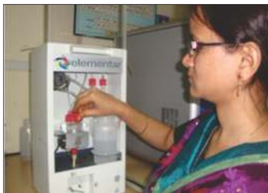
Fig 13. Handling of TOC analyzer for estimation of total carbon and inorganic carbon
