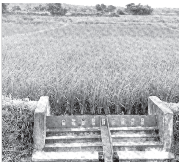
Plate 1 : Experimental plot for determining optimum weir height for in-situ rainwater conservation
