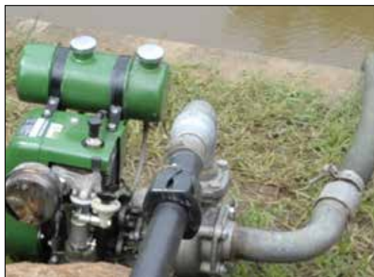
Fig.4 Portable diesel pumpset of 1.5 hp
