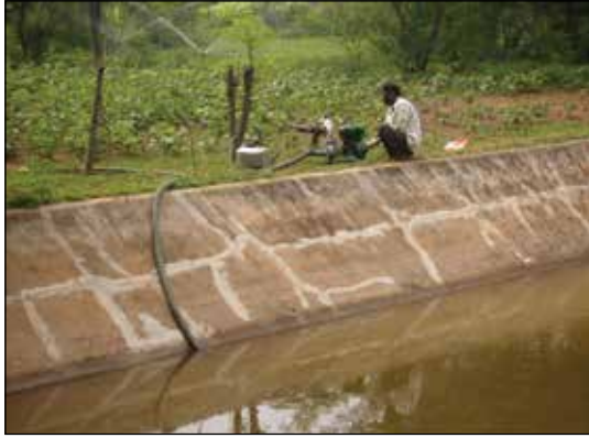
Fig.5 Lifting of water through portable pump set and irrigation to crops near by pond
