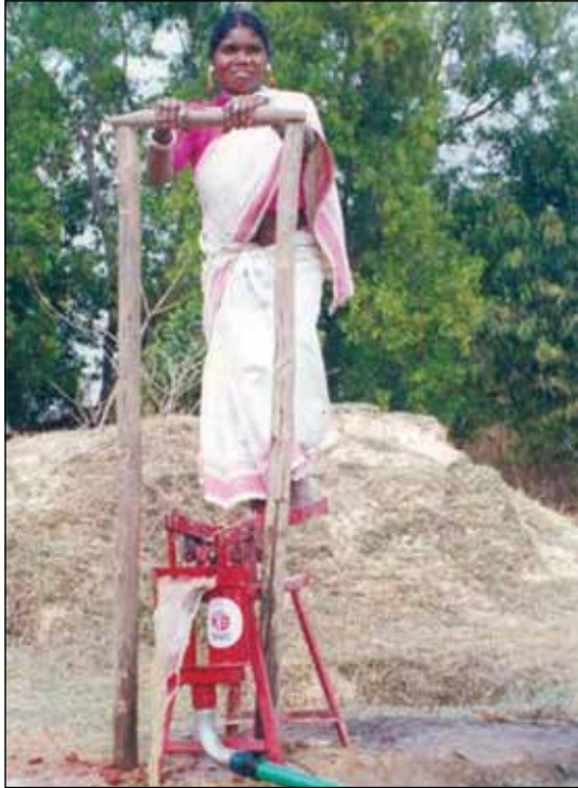
Fig.2 Pedal operated reciprocating pump
